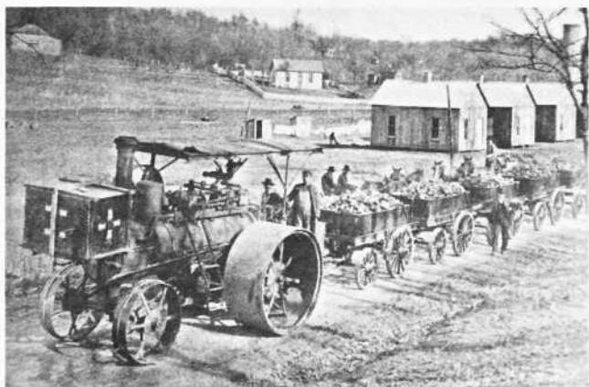
A large steam engine at Burke Brick Company hauling about 7000 bricks to the place where they were to be used. The engine made four trips a day to haul 28,000 bricks daily. Courtesy Bob Rice.
