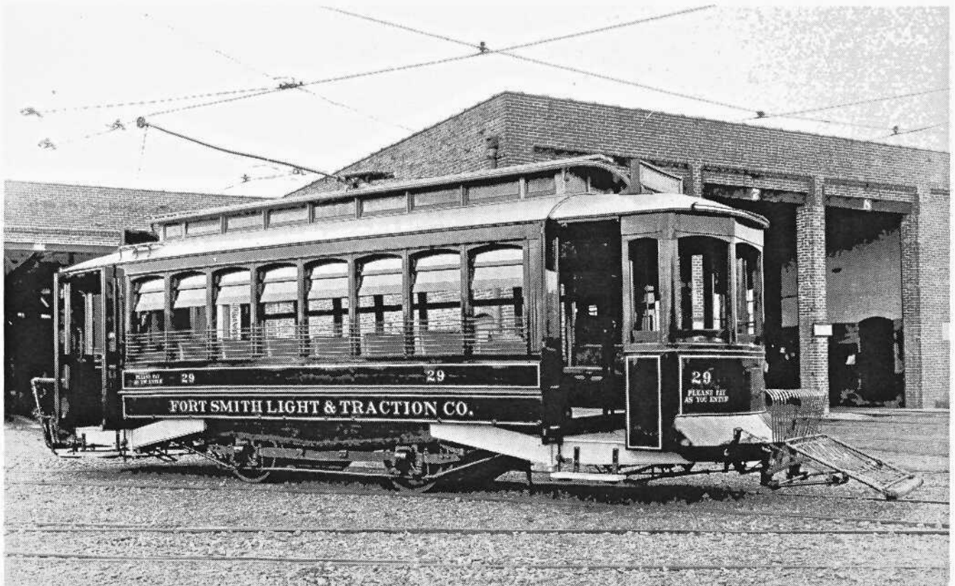
Car #29, built by Danville Car Company in 1910, is 21 ft. 8 in. long semi-convertible car with a Brill truck. This car is a Pay-as-you-enter car.
